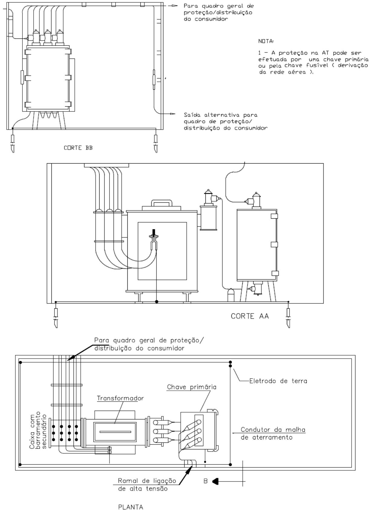
**FIGURA 24 CAMARA MODULO II**
