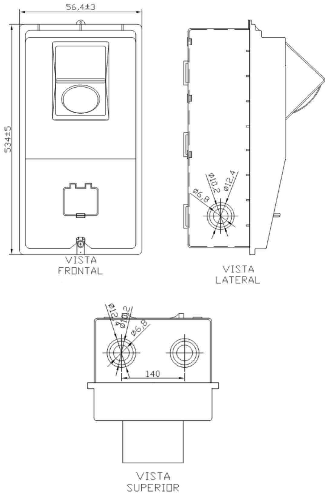
**FIGURA 59 CAIXA POLICARBONATO MONOFÁSICA LEITURA EM POSTE**
