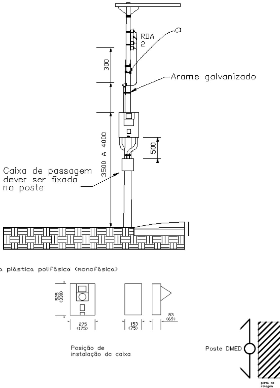
**FIGURA 14 MEDAÇÃO E TOMADA PARA AMBULANTES NOS POSTE METÁLICOS EM AREA CENTRAL**
