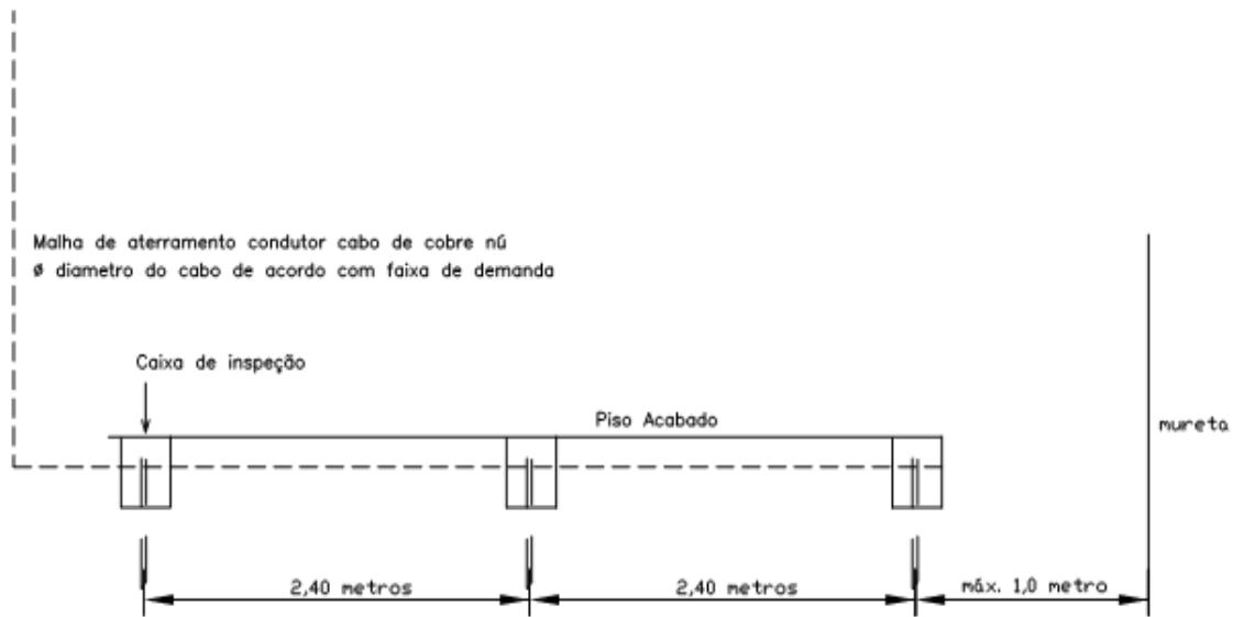
**Haste Cooperweld ou cano de aço galvanizado 1'**
