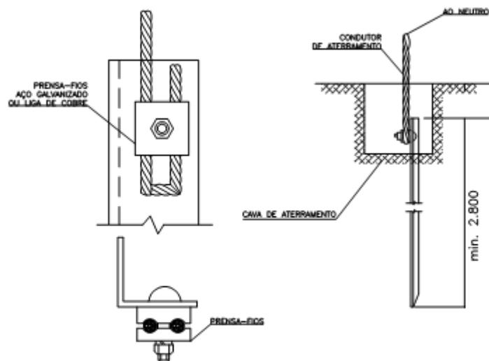
**DETALHE DA CONEXÃO DO CABO
