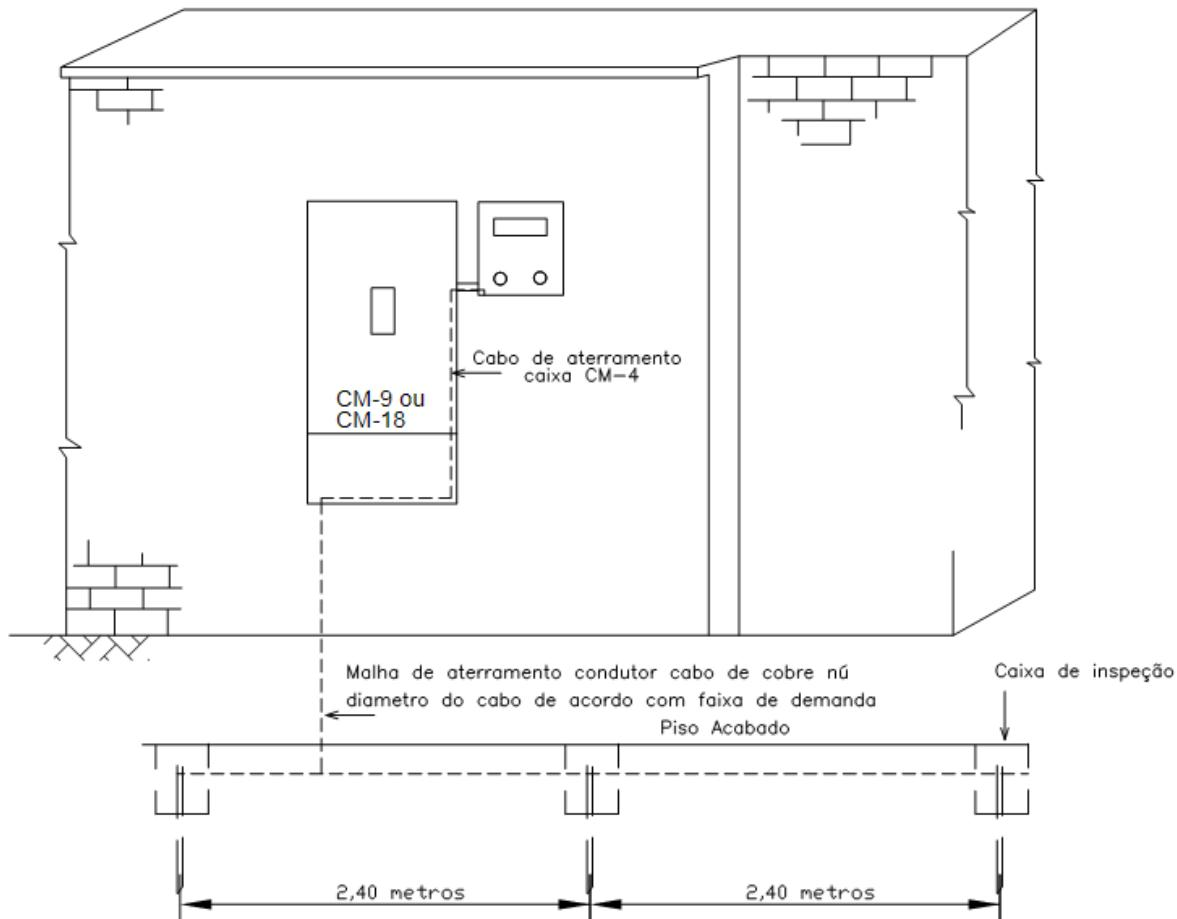
**FIGURA 45 DETALHE DE ATERRAMENTO UC COM CARGA ACIMA DE 34 KW**
