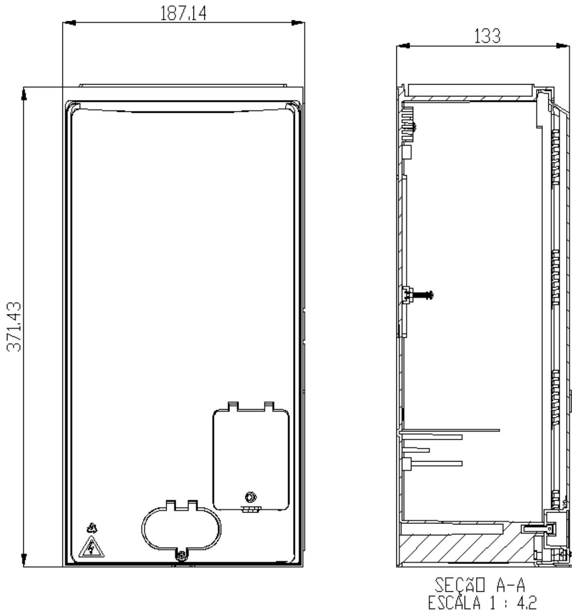
**FIGURA 62 CAIXA POLICARBONATO PARA DISJUNTOR GERAL ATÉ 200A**
